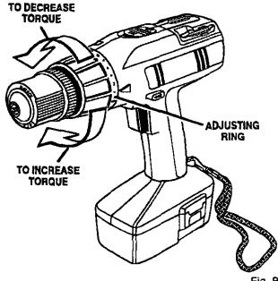
Note: Remember the two-speed feature (HI-LO) when setting torque. The amount of torque will vary depending on which speed setting you have your drill-driver. Switching to LO speed will increase torque. Switching to HI speed will decrease torque.
